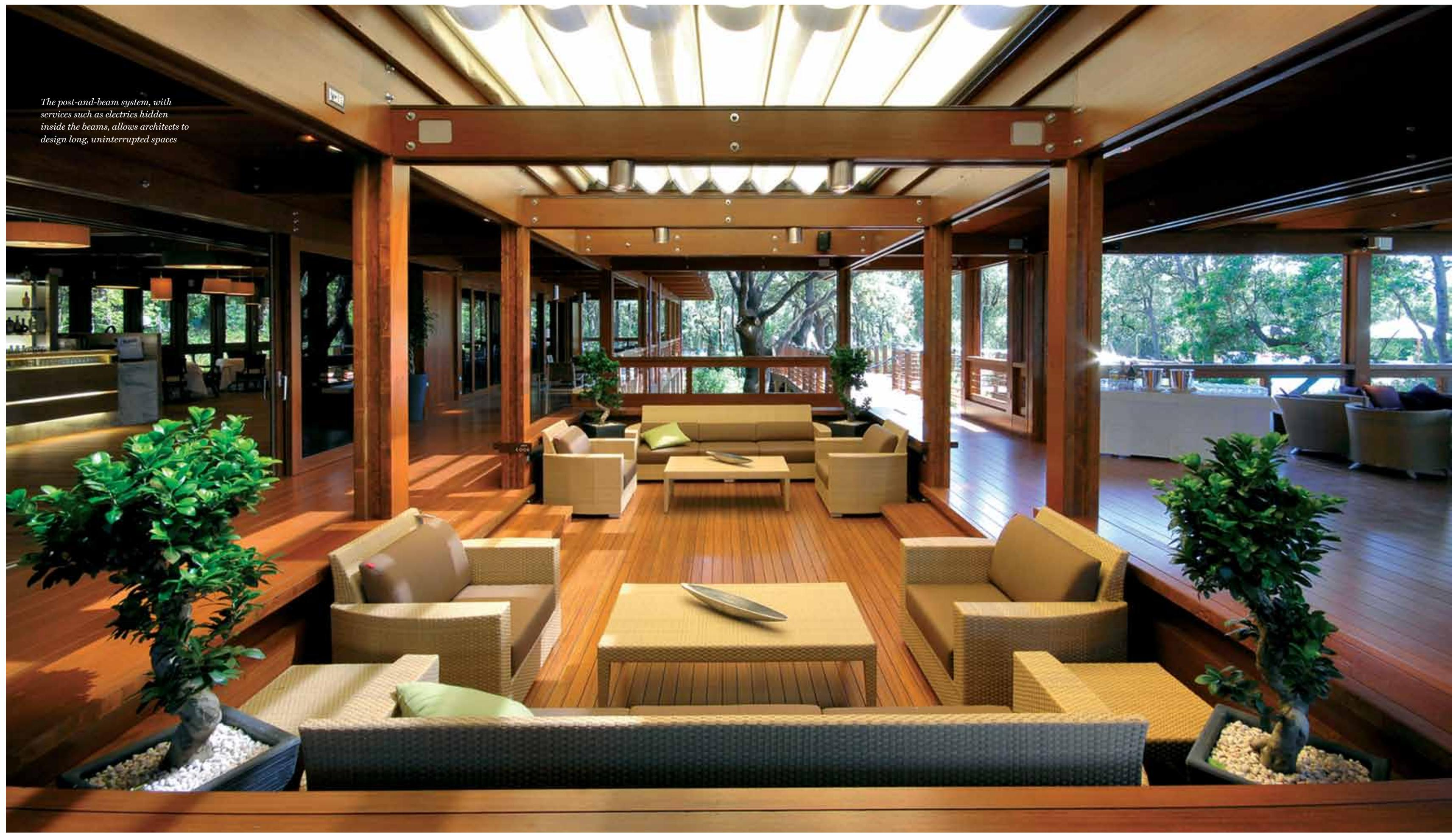
*The post-and-beam system, with services such as electrics hidden inside the beams, allows architects to design long, uninterrupted spaces*
